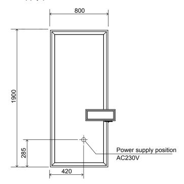
Rated voltageRated frequencyMass230V50/60 Hz70 kg
